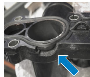
Fig. 3: Breakage (damage pattern)
